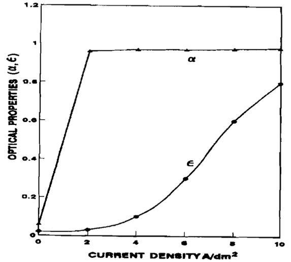
Fig.2: Influence of current density on optical properties ( $\alpha, \epsilon$ ) for an electrolyte containing  $\text{NiSO}_4$  10 g/l,  $\text{CoSO}_4$  10 g/l,  $\text{CH}_3\text{COONH}_4$  10 g/l, 308K, pH 6.2, 30 Sec.
