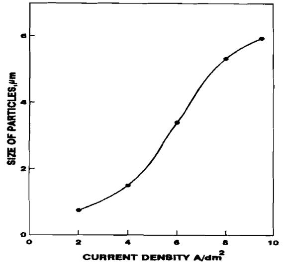
Fig.4: Influence of current density on size of majority of particles of the coating deposited from the electrolyte containing  $\text{NiSO}_4$  10 g/l,  $\text{CoSO}_4$  10 g/l,  $\text{CH}_3\text{COONH}_4$  10 g/l, 308K, pH 6.2, 30 Sec.
