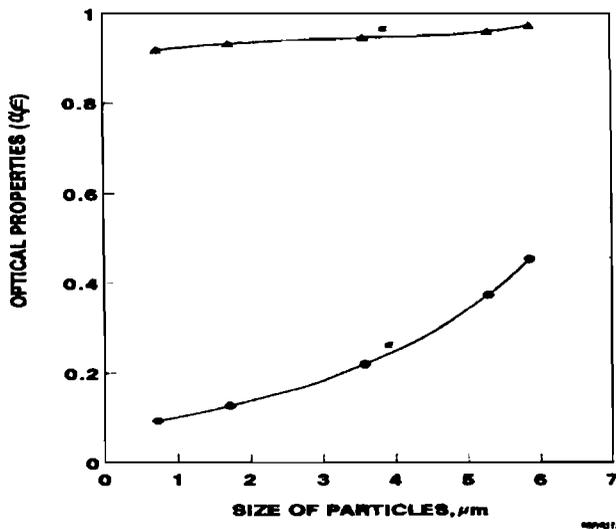
Fig.5: Influence of size of majority of particles of the coating on optical properties (α, ε)
