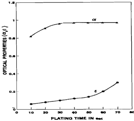
Fig.1: Influence of plating time on optical properties ( $\alpha, \epsilon$ ) for an electrolyte containing  $\text{NiSO}_4$  10 g/l,  $\text{CoSO}_4$  10 g/l,  $\text{CH}_3\text{COONH}_4$  10 g/l, 308K, pH 6.2,  $4\text{A}/\text{dm}^2$ .
