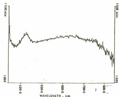
Fig. 2: UV spectrum of doped polyisoprene
