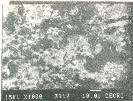
Fig. 1: FeNiMoB-met-glass ribbon without any compression
