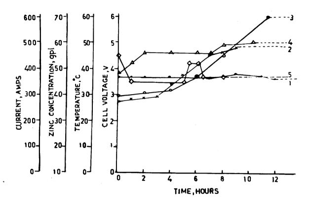
Fig. 1: Variation of cell voltage, temperature, zinc concentration in the electrolyte and current at a fixed applied voltage of 31V. 1. ■ Cell voltage; 2. X—X Temperature; 3. O—O Zinc concentration; 4. △——△ Current; 5. ◇——◇ C.V. in a 1000 amp. cell
