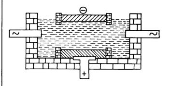
Fig.1 . 3 Layer Cell (Lab Scale) 200 A. without feeding arrangement
