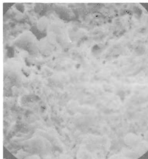
Fig. 17: SEM Fractograph of specimen fractured under slow strain rate in 3.5% NaCl + 0.5% acetic acid + H 2 S (pH = 2.6)
