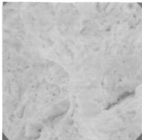
Fig. 13: SEM Fractograph of specimen fractured in 3.5% NaCl + 0.5% acetic acid + H 2 S (pH = 2.6), 40% proof stress
