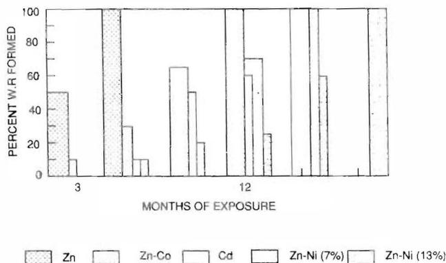
Fig. 1: Marine exposure studies W R on zinc alloys
