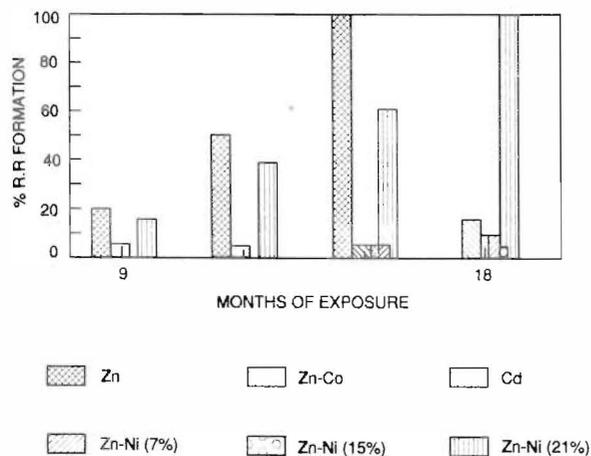
Fig. 4: Marine exposure studies R R formation on passivated alloys
