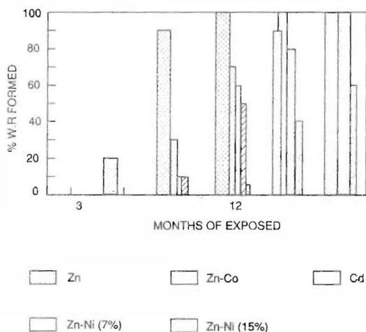
Fig. 2: Marine exposure studies W R on passivated zinc alloys
