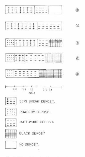
Fig. 1: Effect of zinc chloride configuration in the nickel-tin alloy bath on hull cell pattern
