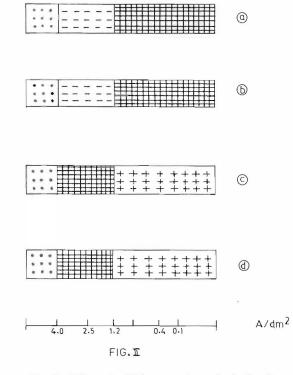
Fig. 2: Effect of addition agents on the hull cell pattern in the nickel-tin-zinc alloy bath (a) Plain bath (b) 1 g/l benzotriazole (c) 1 g/l thiourea and (d) 2 g/l thiourea
